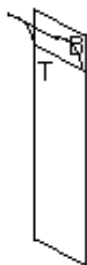
A top, T, tape and a bottom, B tape ready to be pulled apart.
